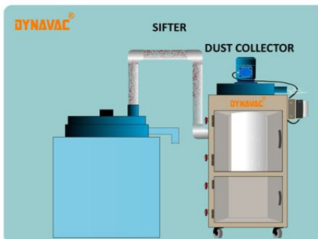
Dust particles collection from sifter during sieving operation
