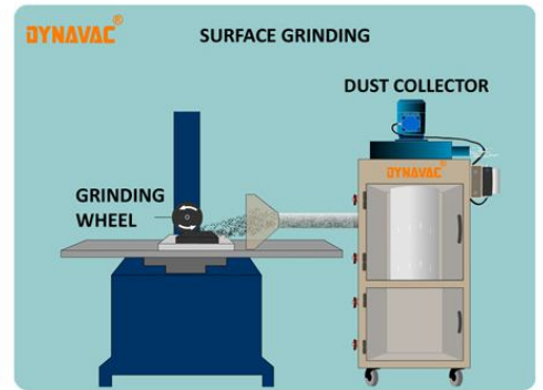
Dust collection from surface grinding operation
