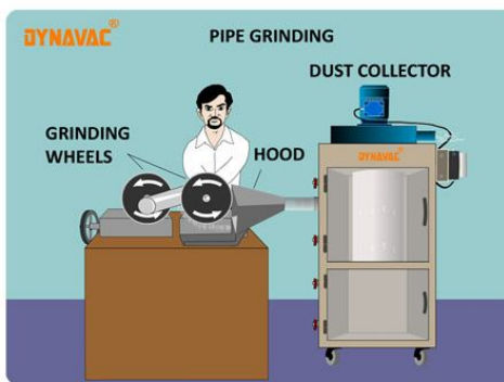
Dust extraction from pipe grinding operation
