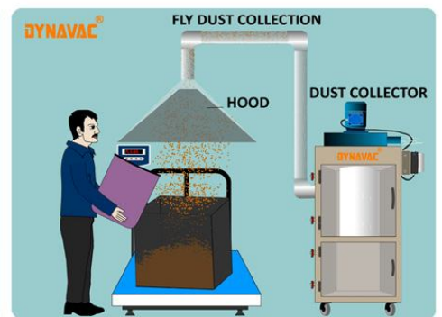
Fly dust collection during product weighing with fixed canopy hood
